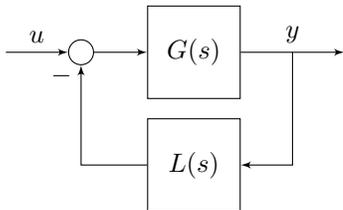
Fig. 1: Block Diagram of General Networked Dynamical Systems
