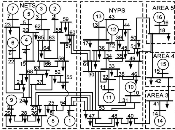
Fig. 5: IEEE 68-bus test system [24]. Image credits to [26]. (NETS: New England test system, NYPS: New York Power System)
