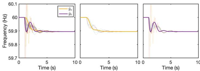
Fig. 6: IEEE 68-bus system (16 generators): Step Response of  $T_{yu}(s)$  and  $T_2(s)$  from algorithm 2. (Middle) Response shown for only group  $a$ , (Right) Response shown for only group  $b$ . The generator injected with step disturbance is in group  $b$
