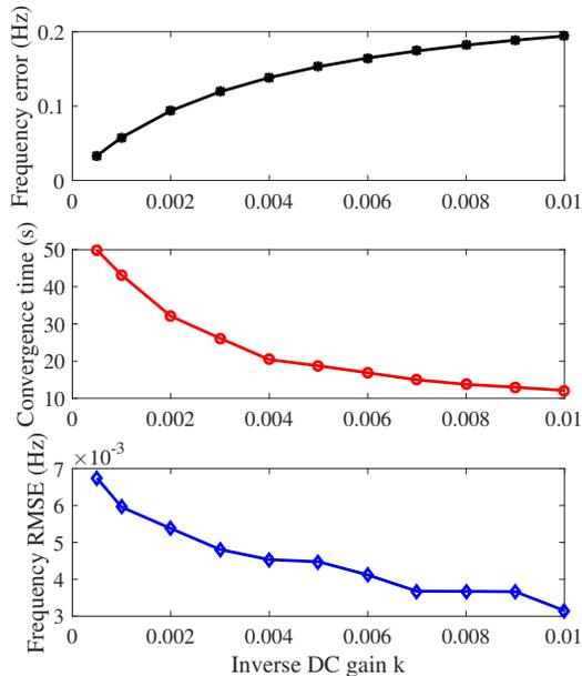
Fig. 5. Steady-state error (upper), convergence time (middle), and RMSE (lower) of frequency at generator G1, as functions of the gain  $k$  for leaky integral control. The time constants are  $T_i = \tau = 0.05$ s for all generators.
