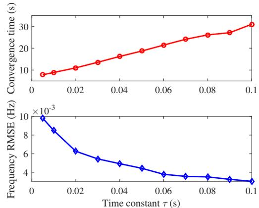
Fig. 6. Convergence time (upper) and RMSE (lower) of frequency at generator G1, as functions of the time constant  $T_i = \tau$  for leaky integral control. The gains  $K_i$  are 0.005 for G3, G5, G6, G9, G10 and 0.01 for other generators.
